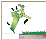
The rod rearms automatically with the simple lifting of the implement.
