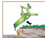
The Shock Control goes into action and disarms the rod.
